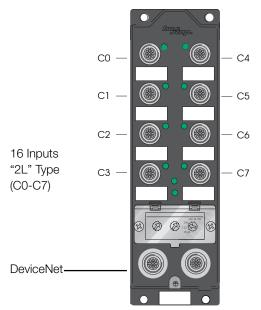
This *busstop*<sup>®</sup> station takes in up to sixteen discrete three-wire inputs or eight discrete four-wire input points per node. There are two inputs per connectorone on pin four and one on pin two. Each input automatically detects a sourcing (PNP) or sinking (NPN) open-collector signal. Any combination of NPN and PNP devices may be used.
